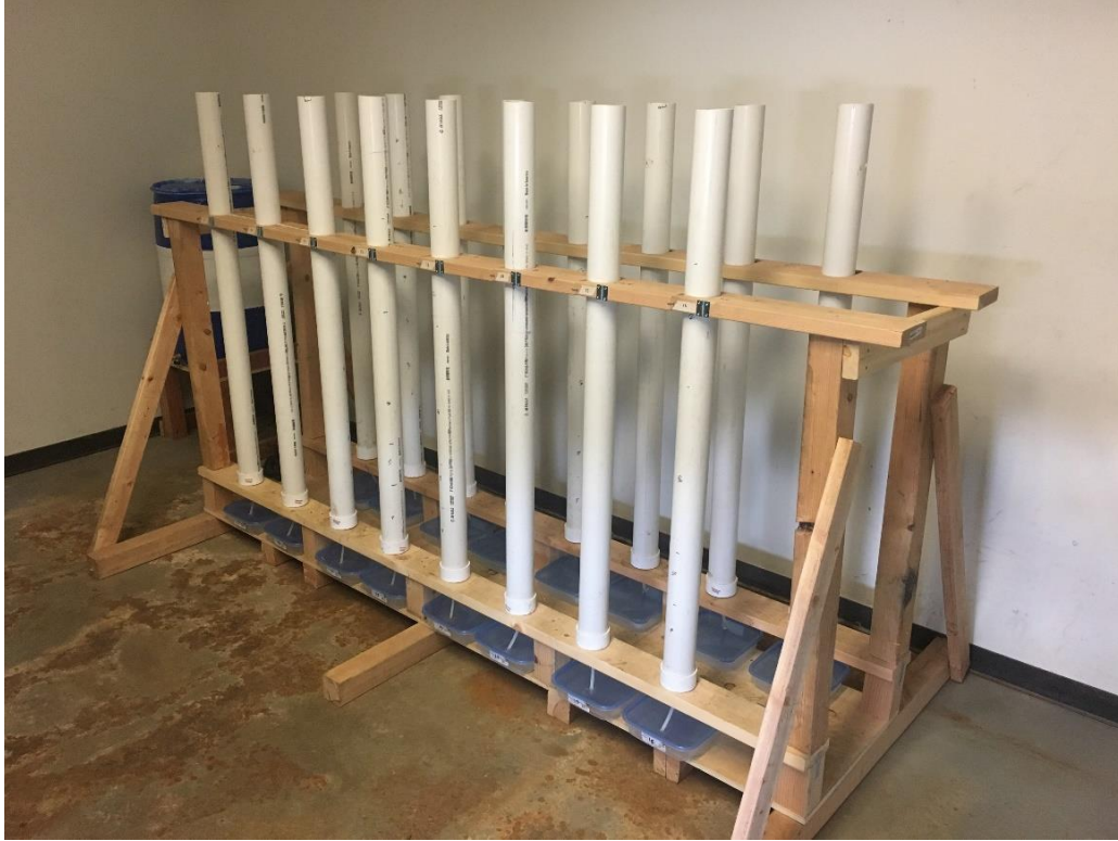
Figure 7: Support structure for columns containing filtration mixtures. Covered effluent catchment containers were placed below each column.
