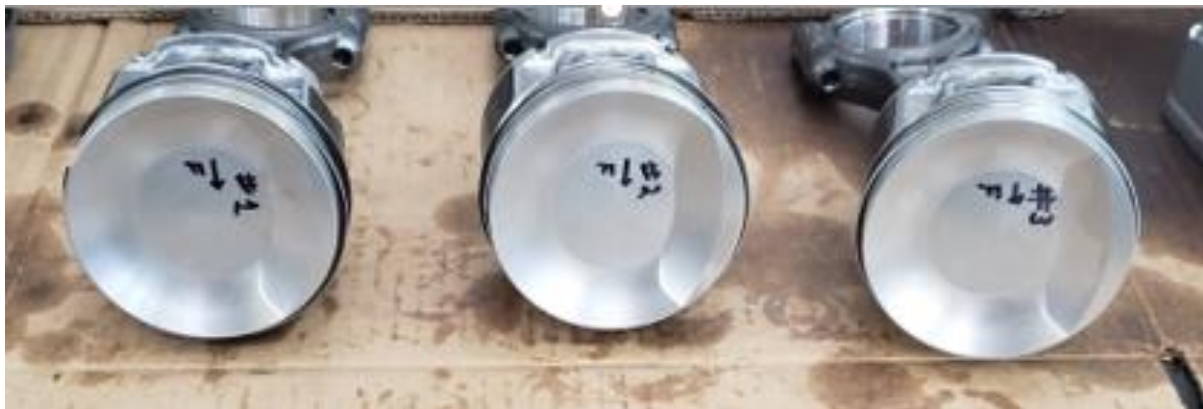
Figure 36. Modified 17:1 Pistons Ready for Installation
