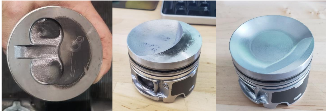
Figure 35:a) Stock Diesel Piston b) 21:1 Piston, c) 17:1 Piston
