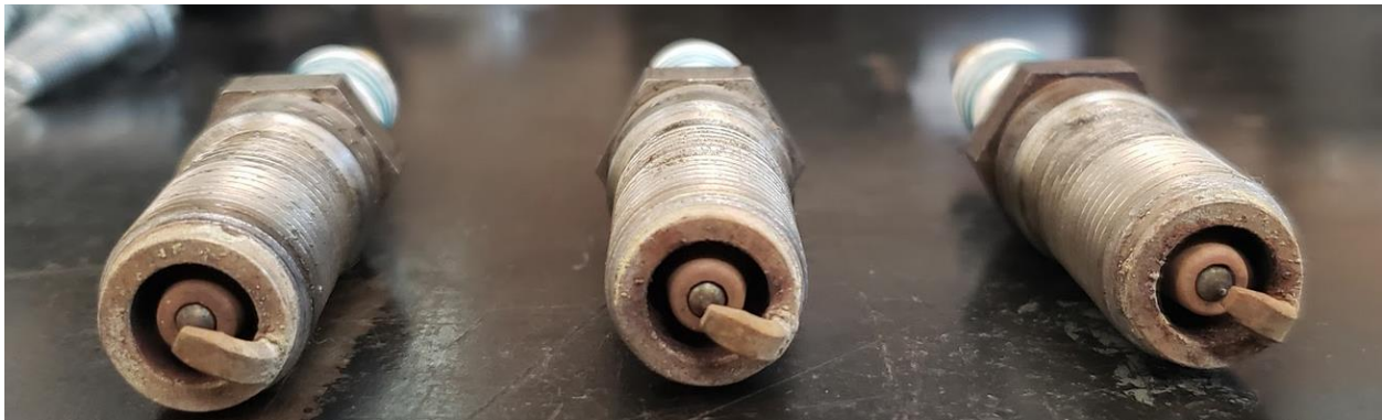
Figure 86: Cylinder 1 through 3 Spark Plug Deposits
