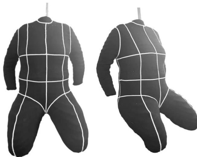
Figure 4.14: Finished half-scale dress form based on Hannah 3D body scan.
