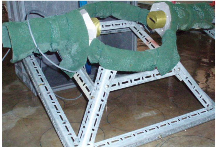
Figure 5. DBS in measurement position, perpendicular to average droplets path, wrapped with anti-projection coating
