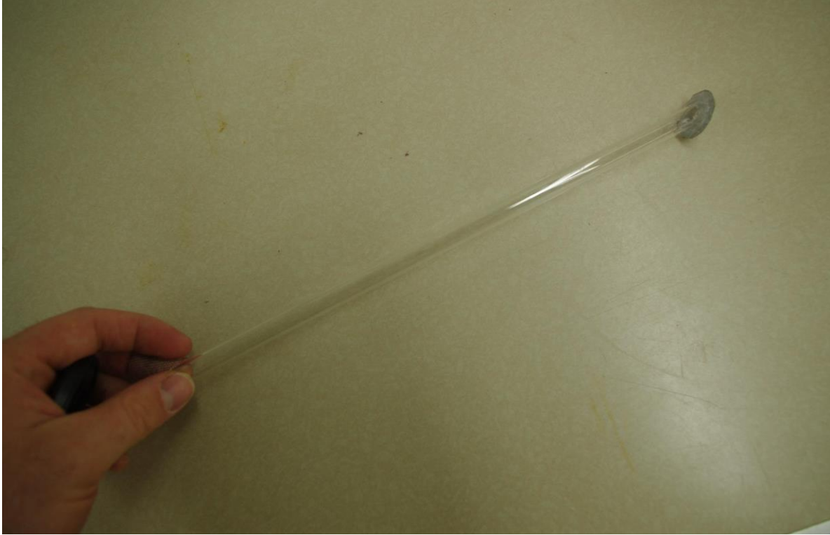
Figure S4.2 Exposure tubes. Aquarium-grade silicone was used to affix stainless steel mesh (105 x 125 micron pore size) to the beveled (30°) end of 24 borosilicate glass tubes (8 mm I.D., 12 mm O.D., 27 cm long). These tubes retained mid- and first-instar age classes during exposure and enumeration. Small strips of fine mesh (3 x 30 mm) were placed inside each tube as substrate for the organisms.
