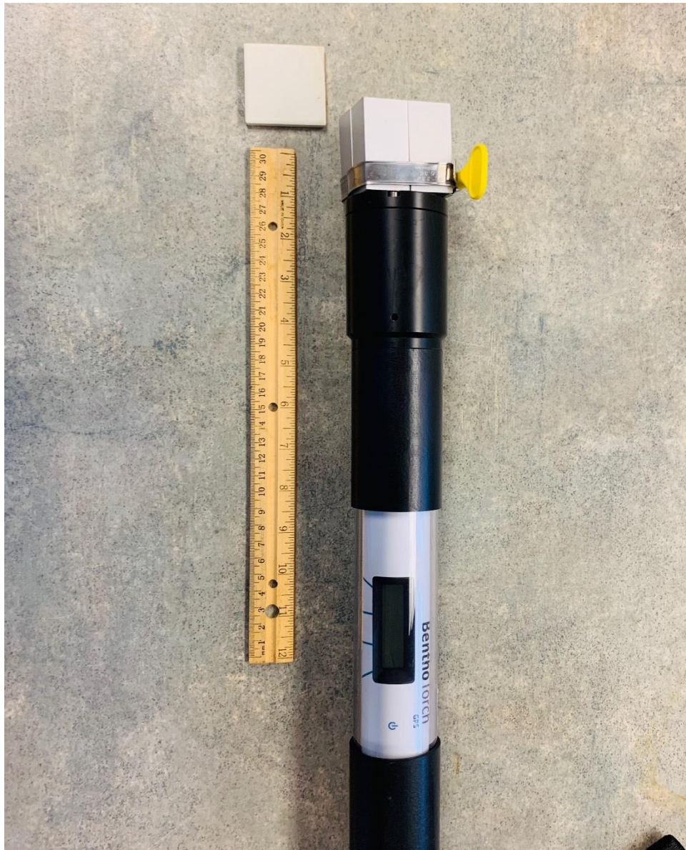
Figure S5.2 Photo of Benthotorch tile adapter used to estimate algal biomass and community structure on different ceramic tile treatments in stream mesocosms. The main purpose of the tile adapter was to reduce sloughing of algae during measurements and consistently sample the same location on each respective tile.
