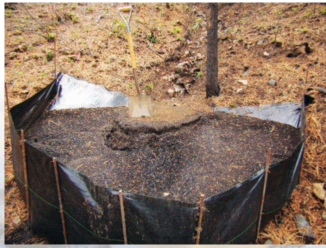
Figure 2. Sediment fence used to measure erosion after the High Park Fire. After rainstorms, researchers dug out and measured the accumulated mass. These are placed in small convergent hillslopes as indicated by the small rill leading into the sediment fence, indicating significant post-fire overland flow. Photo by Sarah Schmeer.
