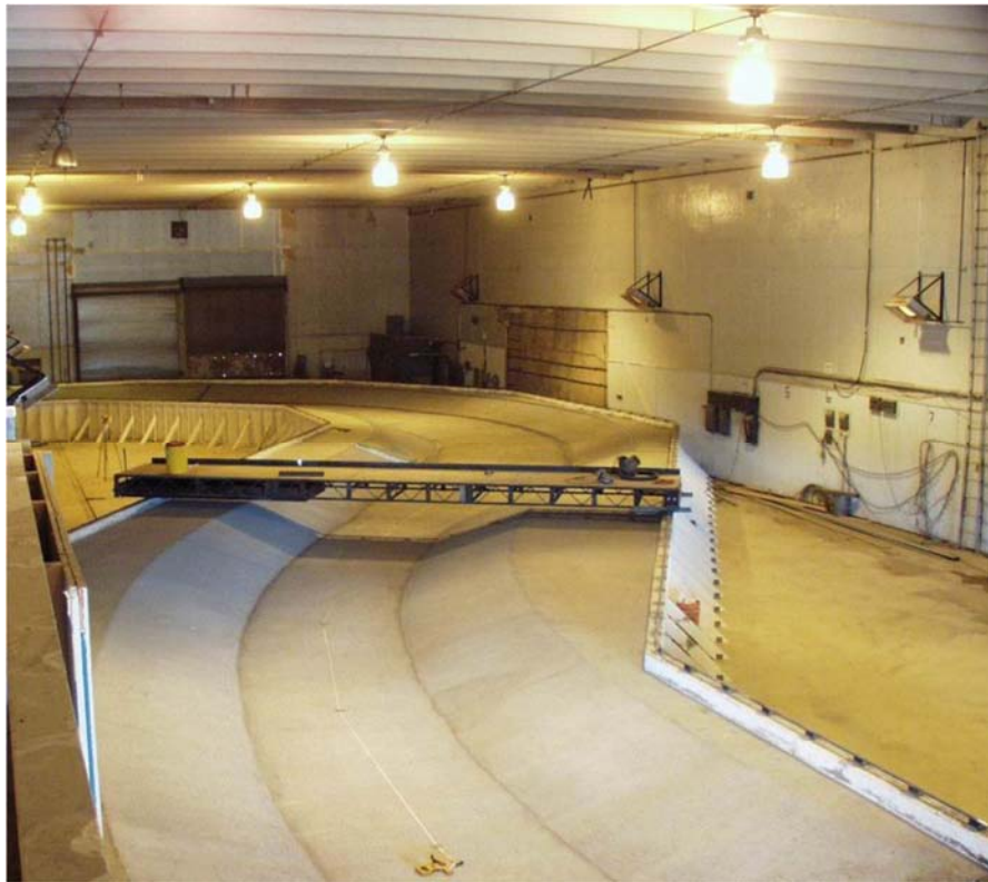
Figure 6: Trapezoidal channel used in the physical hydraulic model (Scurlock 2014)
