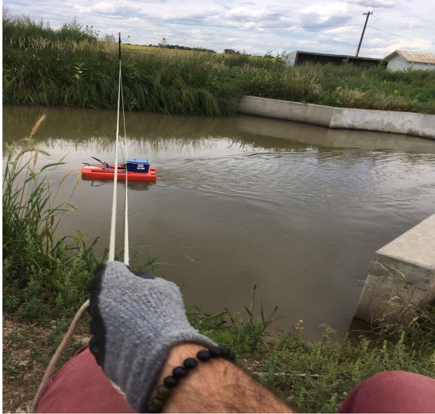
Figure 9. ADCP Operation Mechanism, along the Cross-Section Upstream of Gate C.
