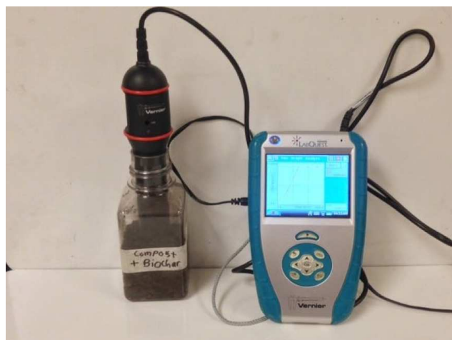
Figure 6.8. Example set up for one experimental treatment replicate for soil respiration classroom investigation using a CO 2 sensor and data collection device. (Credit: Photo by S. Bucko)
