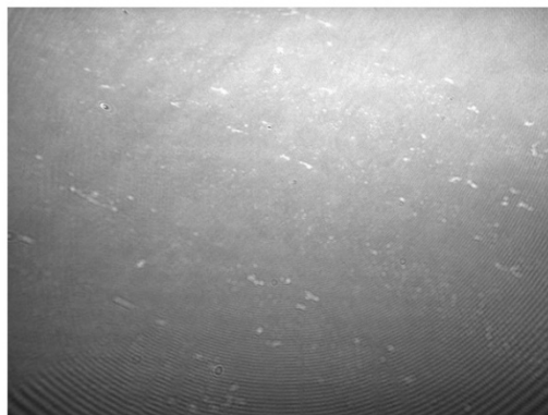
Figure A6.1. BAM images of post compression isotherm collapse of monolayers consisting of 50 nmoles of MK-9. Times post-collapse are given with corresponding images below.
