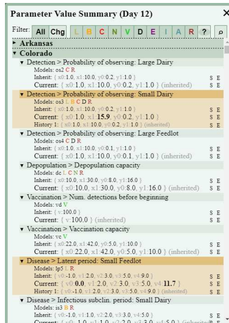
Figure 4.7: The parameter values summary. Users can review prior values, undo changes, and jump directly to each parameter in the menu. Changed entries are highlighted in orange and changed values are bold.
