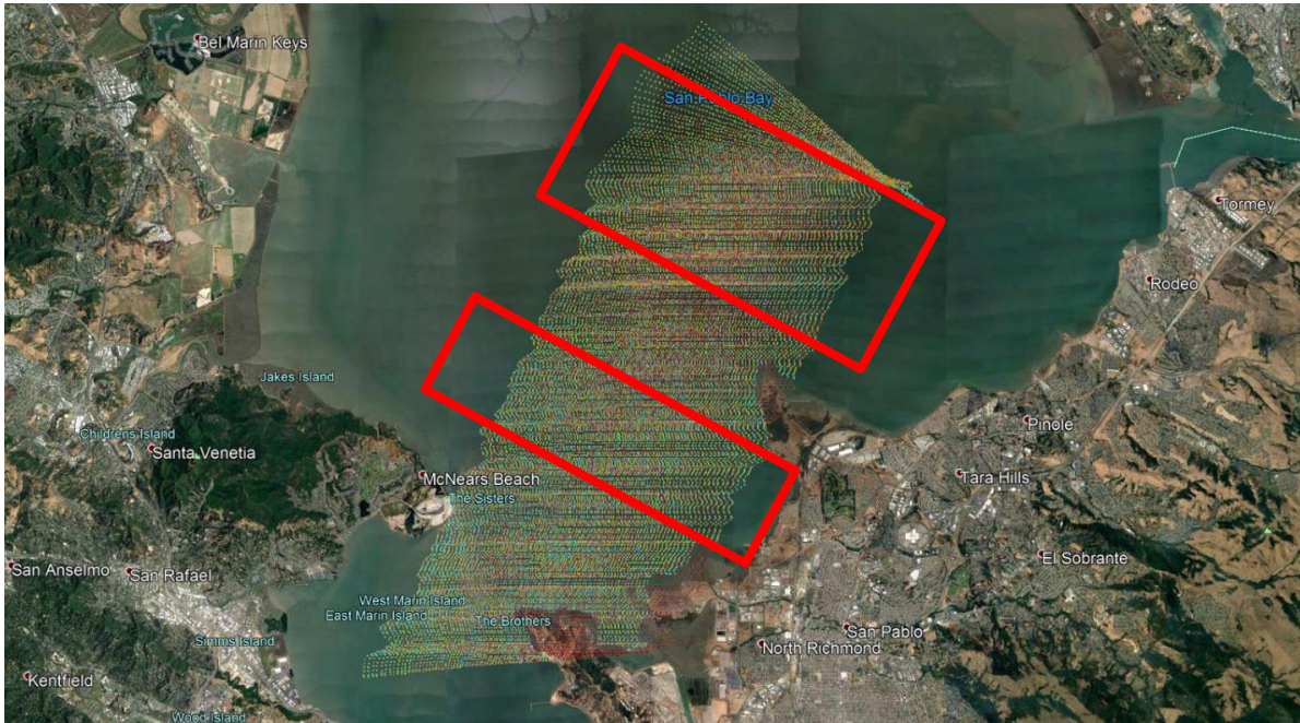
Figure 102: Geo-located antenna temperature measurements of the HAMMR instrument for the WCFC measurements over San Joaquin River. Please note that retrieval valid zones are given in red.
