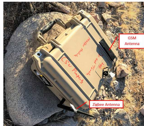
(c) Pelican Case architecture for Master node.
