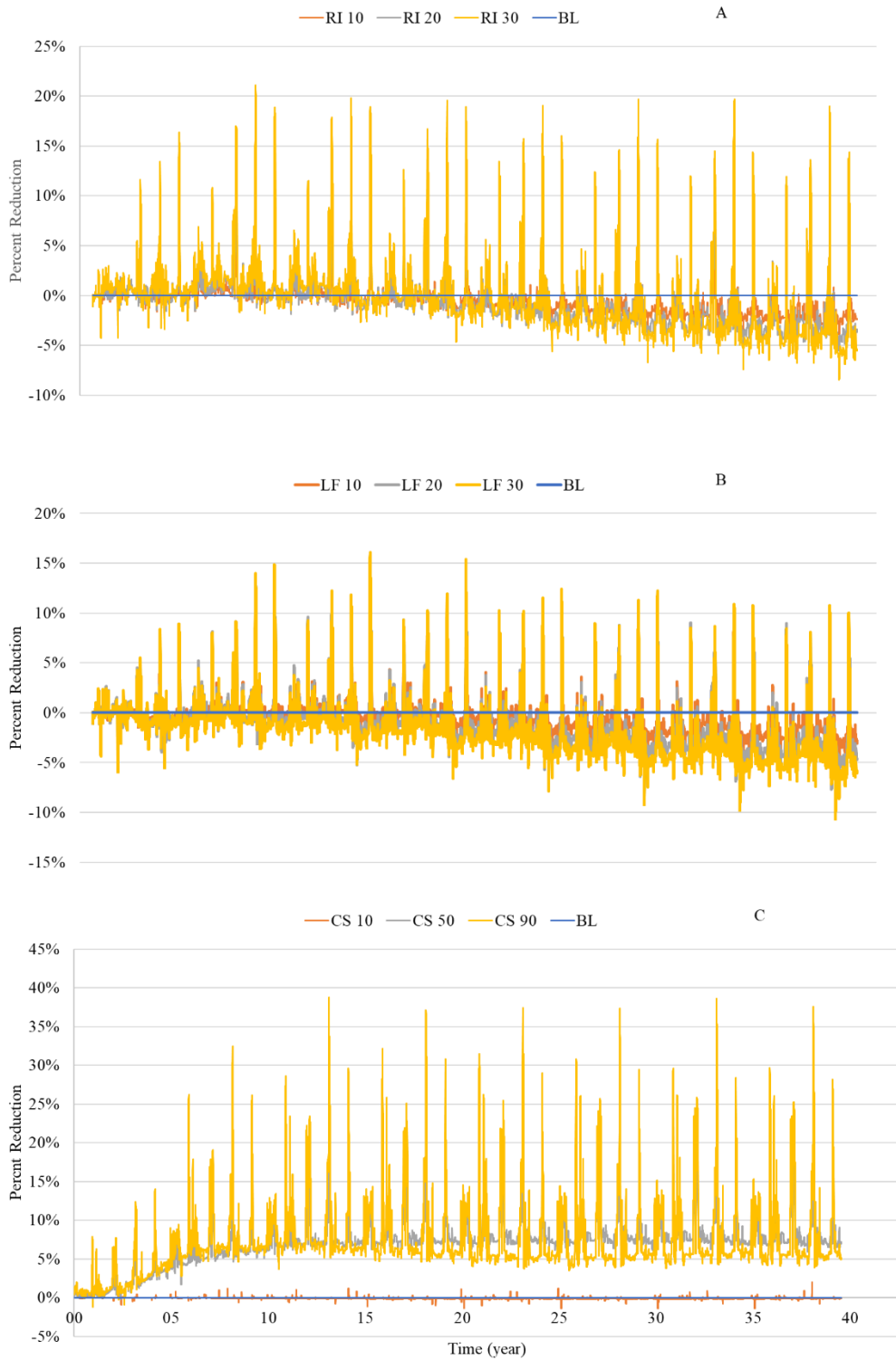
Figure 39 Groundwater concentration reduction for NO 3 over the 40-years simulation (A) reduced irrigation, (B) lease fallowing, and (C) canal sealing compared with the baseline condition
