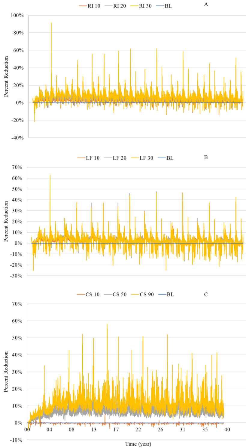
Figure 41 Mass loading reduction for NO 3 over the 40-years simulation - (A) reduced irrigation, (B) lease fallowing, and (C) canal sealing compared with baseline condition.
