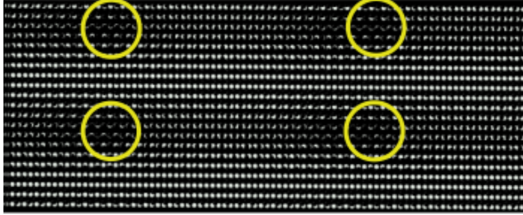
Figure 2.9: Example of O-points (highlighted by yellow circles) in the Bagaryatskii OR. These points were visualized by overlaying the appropriately oriented lattices of ferrite and cementite.
