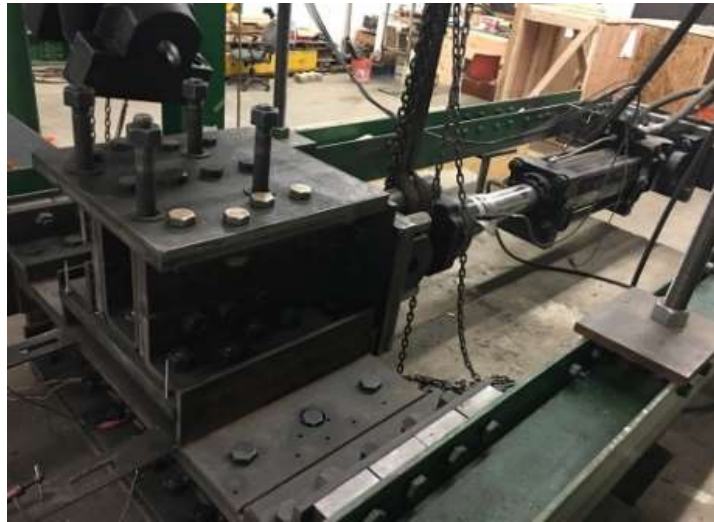
Figure 3-9 Setup For Loosening Test
