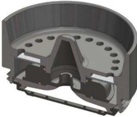
Figure 5-4. Section view of PM 2.5 cyclone.
