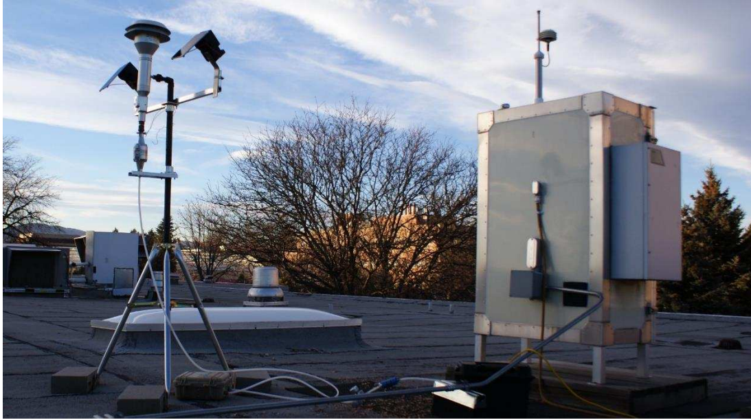
Figure 2-7. Two SPARC samplers mounted with an FRM for a co-location test.
