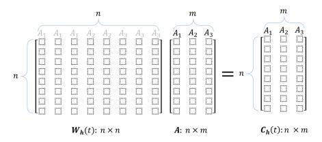
FIGURE 5.2. Depiction of the *h*-hop Adjacency Matrix  $\mathbf{W}_h(t)$  and the Parentto-Child *h*-hop Class Adjacency Matrix  $\mathbf{C}_h(t)$
