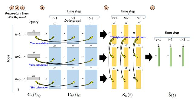
FIGURE 5.3. Graphical depiction of baseline INSiGHT algorithm. This graphic depicts the basic steps in the INSiGHT algorithms described in [144]. Here n' is the number of nodes in the query graph Q, n is the number of nodes in the data graph G, and m is the number of classes. The steps shown are only for the construction of the parts of  $\mathbf{S}_h(t)$  that correspond to the Parent-to-Child class membership similarity; the steps for the Parent-from-Child portions are not depicted.
