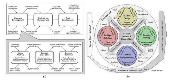
FIGURE 1.1. (a) Principle stages of the systems engineering life cycle with the expansion of concept development phases [174]. (b) Systems Decision Process [239].
