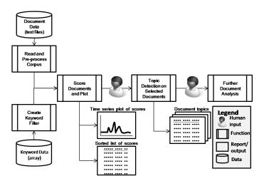
FIGURE B.5. Functional decomposition of the topic detection system.
