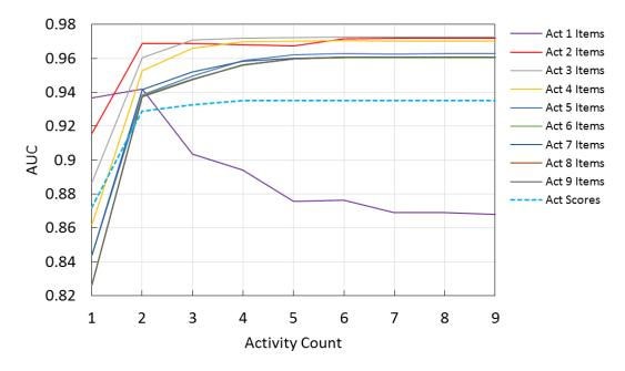
FIGURE 6.7. AUC performance of stepwise logistic regression models on activity sets of various sizes.
