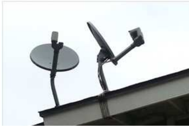
Fig. 19. An image that should be familiar to most people since it is of a satellite TV dish pointed to a geosynchronous satellite.
