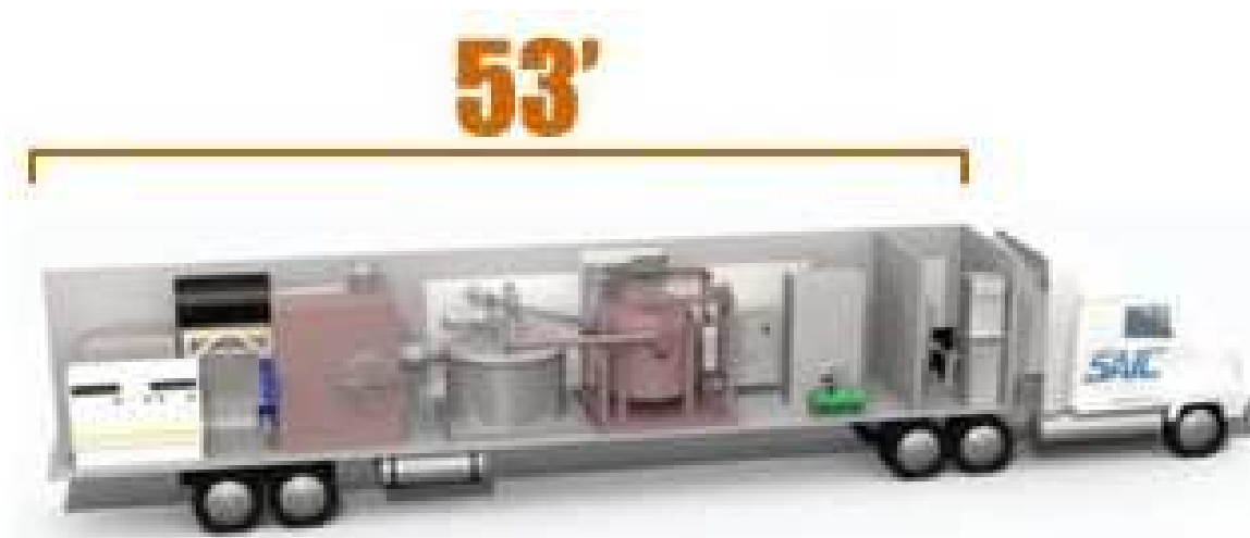
Fig. 10. Image of a transportable pyrolysis system (Courtesy of Trio Renewable Gas, Inc.).
