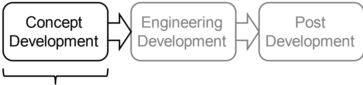
Fig. 1. Major steps in the systems engineering process consist of Concept Development, Engineering Development, and Post Development. Our focus in this work is on concept development and for the SoS described in Chapter 5 the SAI method is used (After [15]).
