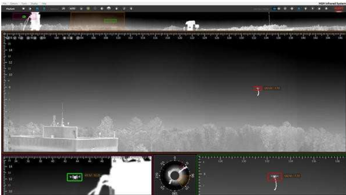
Fig. 42. Infrared camera image of a drone taken using the Cyclope system from HGH Infrared ( http://www.hgh-infrared.com/News/Press/Eyes-on-the-Horizon )
