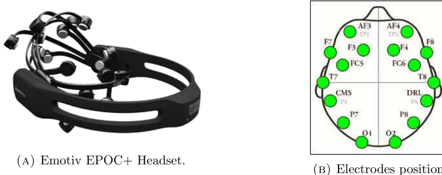
FIGURE 2.7. Emotiv EPOC+ headsets and its electrodes location
