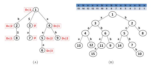
FIGURE 6.3. An example of position heap tree. (a) Constructed from the text "ab\$aaa\$bb" exatracted from documents  $(D_1, D_2, D_3)$ . (b) Constructed from the text "abaaababbabaaba".
