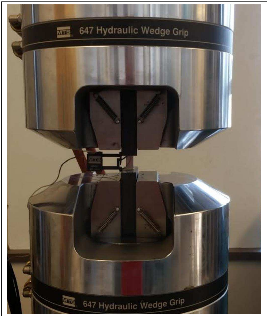
Figure 33: MTS Tensile Testing Apparatus with Extensometer
