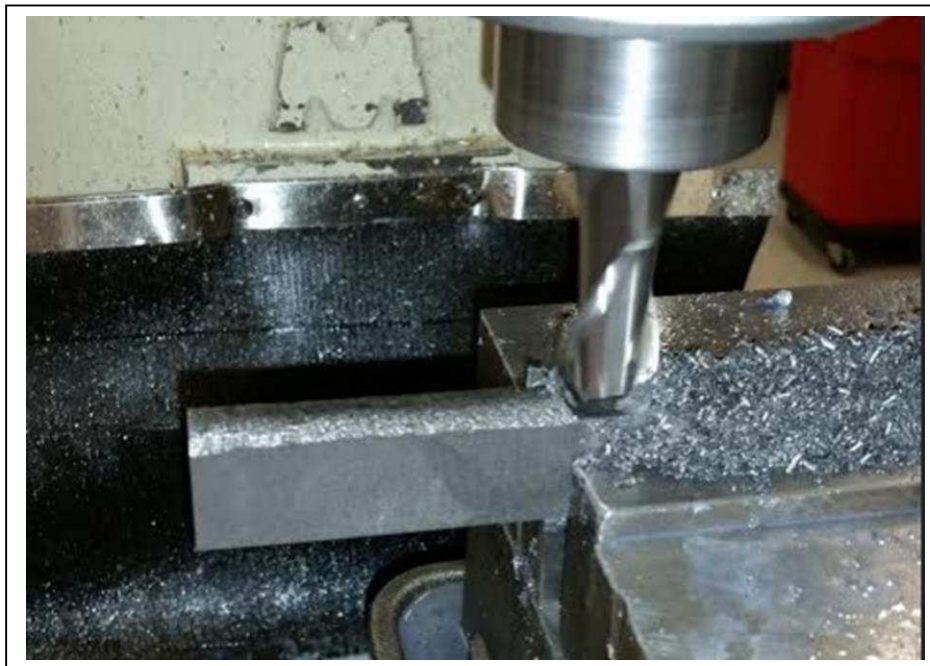
Figure 31: Milling Sample into Rectangular Cross Section
