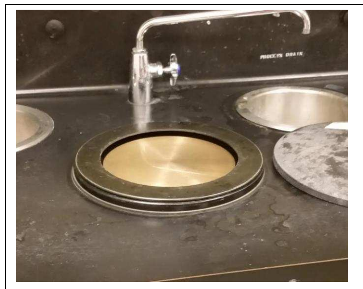
Figure 20: Grinding and Polishing Wheel
