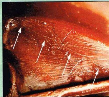
Above: If damage in upper view is not repaired, crack will extend into crankcase webbing in front of main bearing cap (See arrows).
