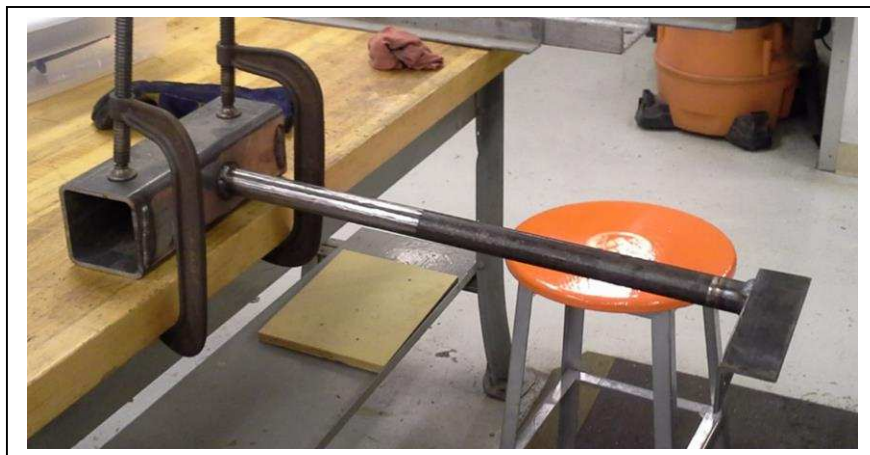
Figure 51: Torsional Cantilever Beam Apparatus
