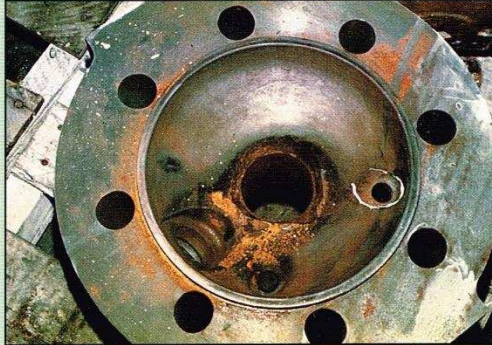
GMV cylinder head damaged in gas valve hole and spark plug area.
