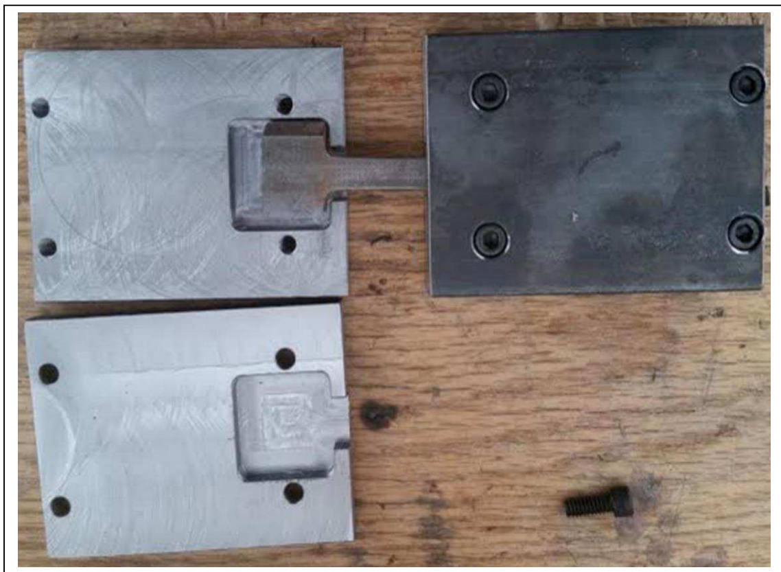
Figure 32: Micro Dogbone Sample and Jaw Adaptors
