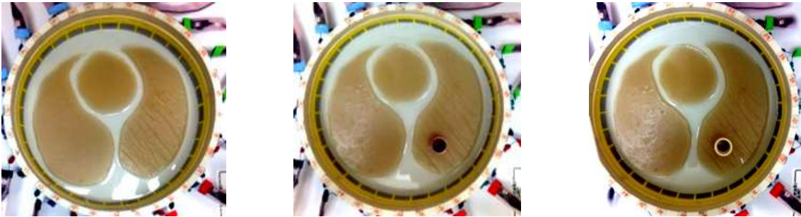
FIGURE 3.16. Left: experimental set-up with agar heart and lungs in a PVC tank, surrounded by saline solution. Middle: a second experiment, in which the heart and lungs are preserved, but a copper conductor has been inserted into the bottom of the right lung. Left: a third experiment, in which the conductor has been removed, and a plastic insulator has been inserted in its place.
