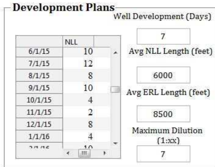
Figure 3-17 The display panel for the development plan in the Water Quality Tool. The number of wells and the drilling data are entered into the Excel spreadsheet by the user. The normal lateral length (NLL) and extended length (ERL) are entered by the user into the tool.
