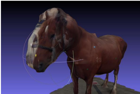
Figure 4.4. Poorly-constructed 3D image of the head and neck of a P group horse. 3D imaging error was induced by subtle movement of the horses during the 2D imaging. In figure 4.4.a, subtle horizontal head movement induced error in the constructed 3D image. Neither the horse handler nor the photographer recognized the horse movement at the time of 2D imaging because the movement was so subtle, but recognized it only after the photogrammetry was finished. In consequence, the constructed 3D image of the head and neck was larger and distorted compared to the true head (Figure 4.4.b and 4.4.c).
