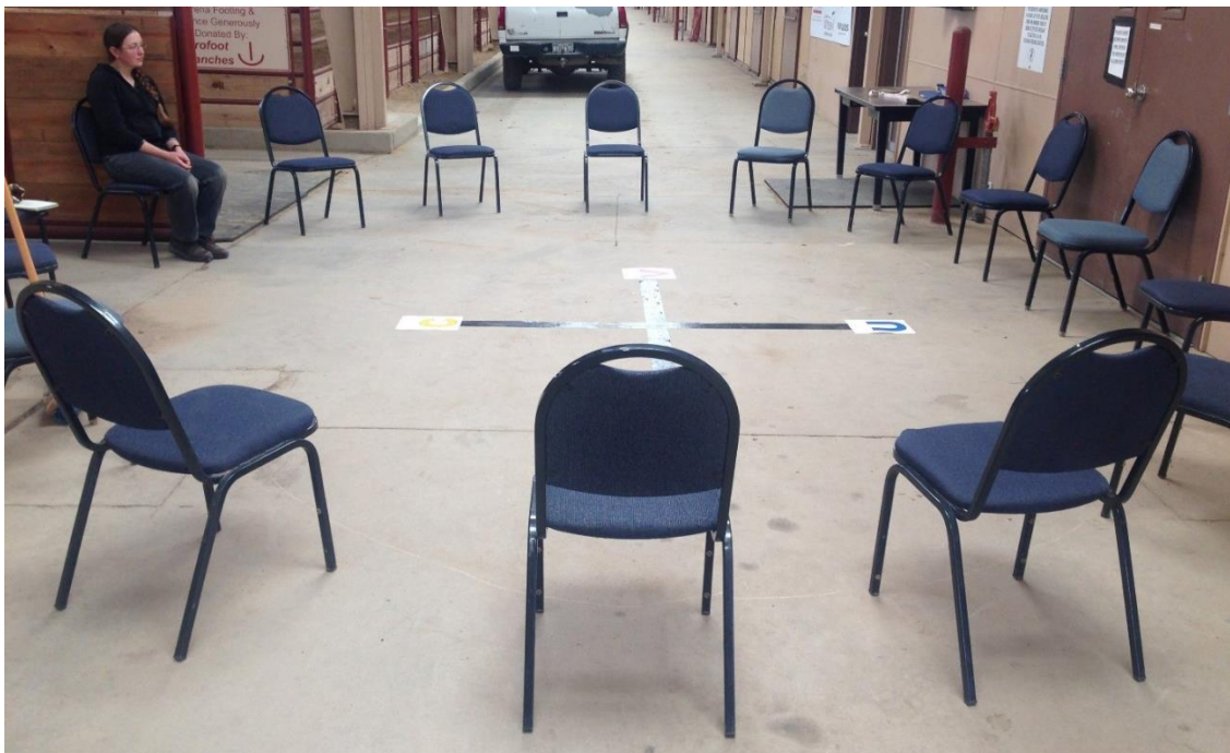
Figure 4.1. The preparation of the location of photogrammetry application. Two linear black reference markers were placed crossing each other on the floor of the study area (Figure 4.1a). The length of each marker was 180 cm. At the ends of the black markers a paper sheet with letters C, S, U, and V, were placed (Figure 4.1.a). To obtain photographs of group P horses, 16 chairs with a seat height of approximately 50 cm were placed to surround the area where the horse stood (Figure 4.1.b).
