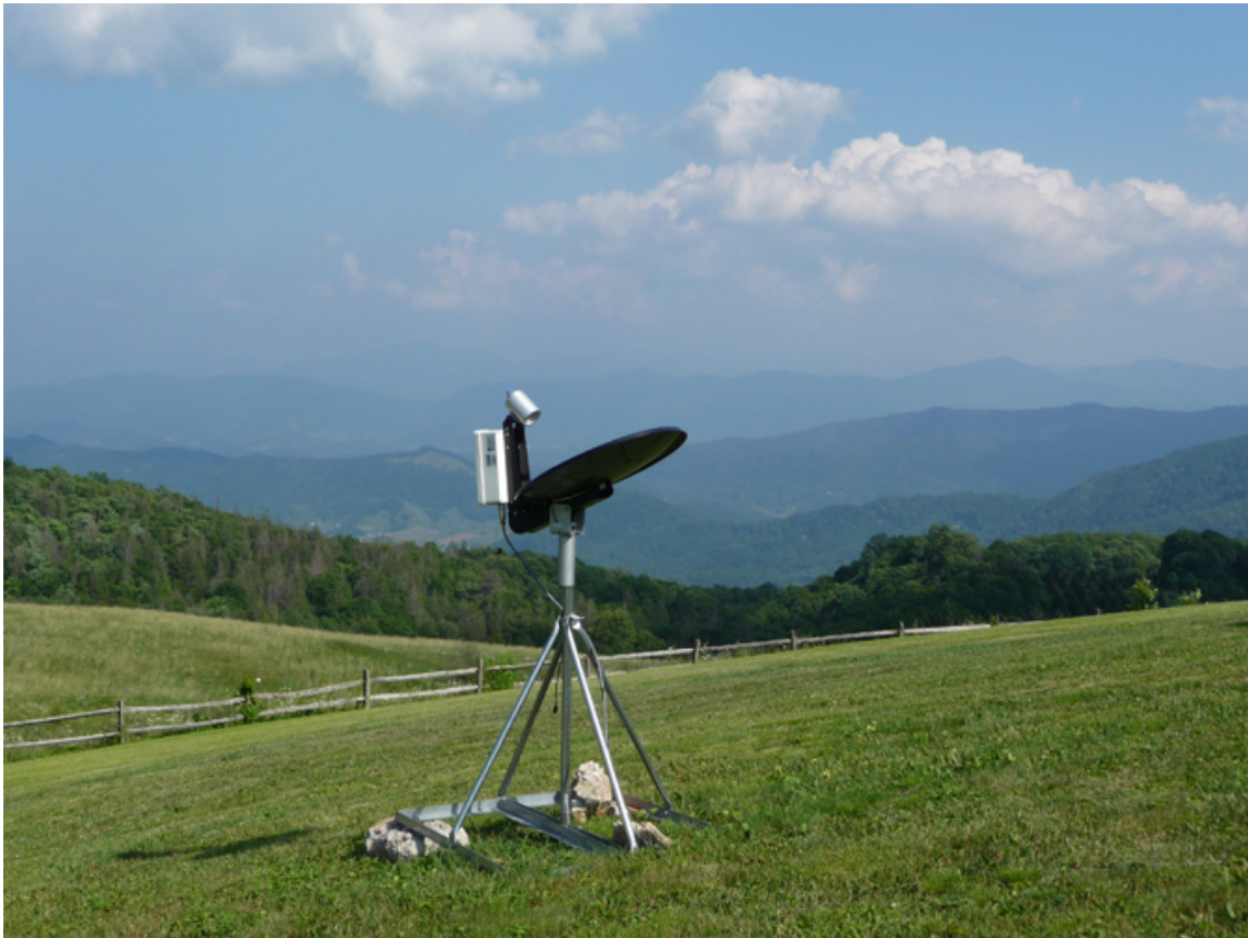
FIGURE 8.15. Micro Rain Radar pictured around Purchase Knob in the Great Smoky Mountains National Park, is a vertical profiler radar that delivers information about vertical structure in the atmospheric column and provides an estimation to the vertical distribution of rainfall. It can operate 24/7.
