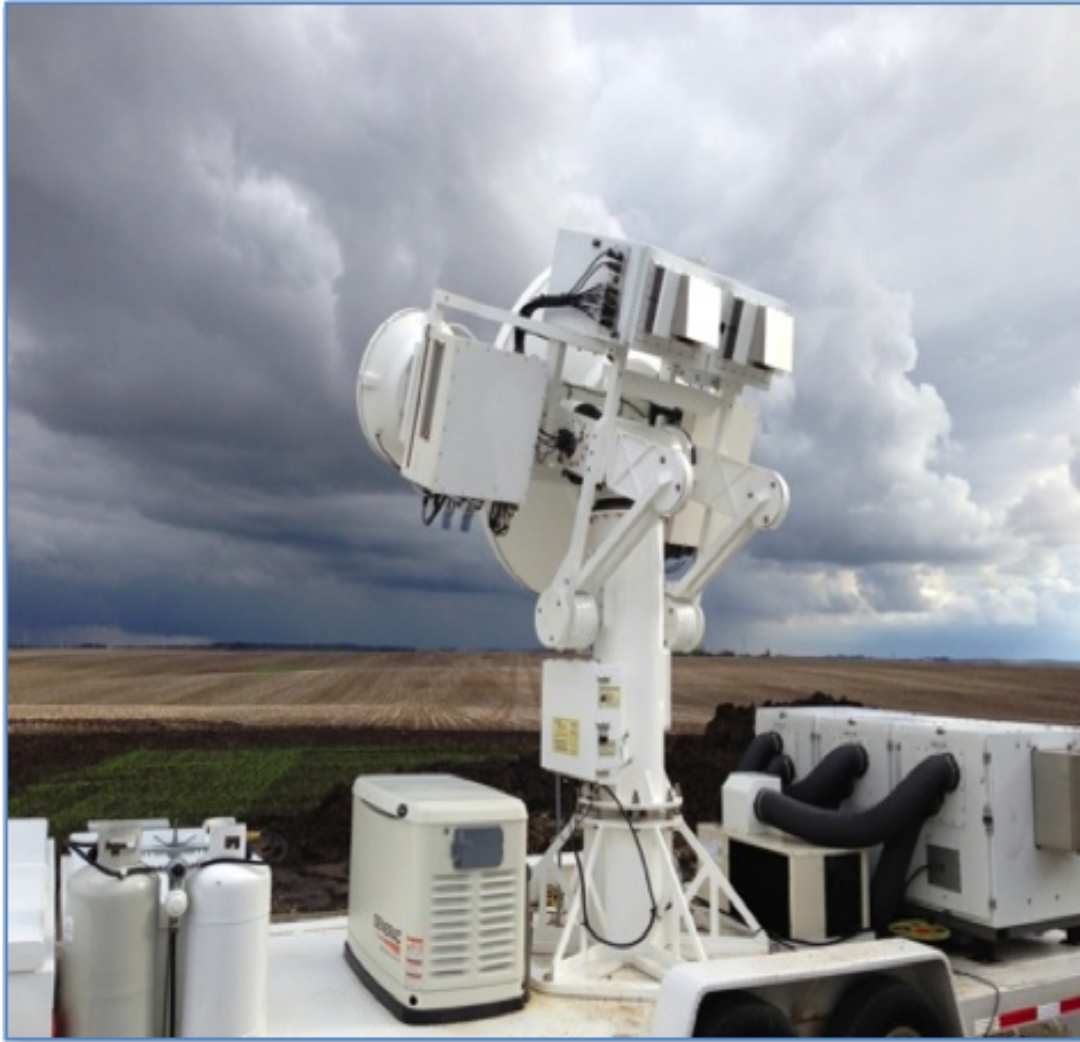
FIGURE 8.11. NASA D3R Ku/Ka band radar operating during the IFLOODS campaign in Iowa.
