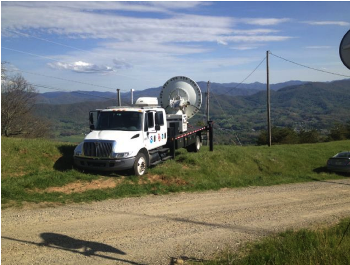
FIGURE 8.12. NOAA NOXP mobile radar on Lookout Mountain overlooking the Pigeon River watershed.
