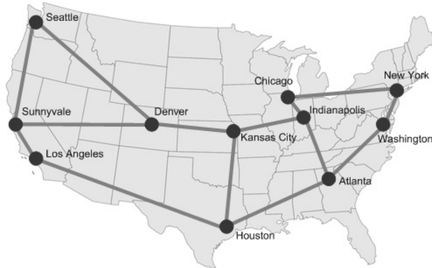
FIGURE 6.16. The Internet2 network [2], consisting of 11 nodes and 14 bi-directional links.
